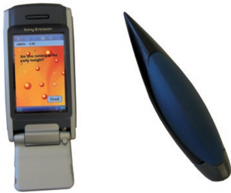
Figure 3.3-2 The eMoto system: a Java application running on a mobile phone plus the extended stylus.
